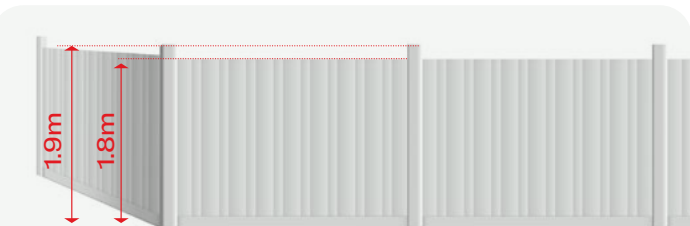
- Diagram 6.1.5a – Corner Fence Elevation
